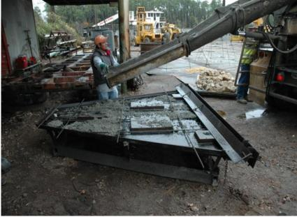
Each mold is poured and a full yard of concrete is used for each Reef.
