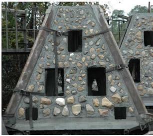
After welding, metal forms are attached to the 3 corners and additional concrete is poured, secured and allowed to cure. Once the reef is cured, it is removed from the brace and is ready for deployment.
